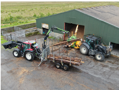
Two Valtras are used by the forestry team to produce woodchip biomass, used for power and heat production. For loading softwood and operating the chipper, the Valtra’s rotating seats are a significant advantage.
